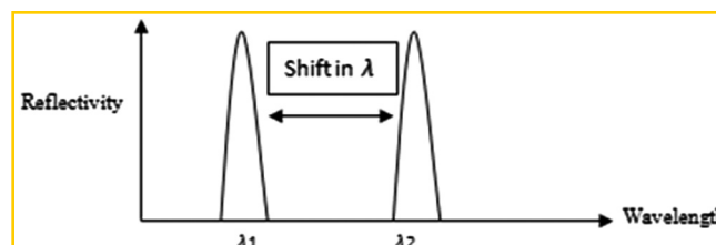
Fig. 7 Wavelength shift due to external perturbation.
